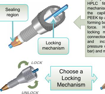
Locking mechanism holds the capillary inside the fitting. Typical HPLC fittings without locking mechanism such as **F-1032** hold the capillary by compressing PEEK tip around the capillary and forming both a seal and a holding force. Having an additional locking mechanism makes the connection much more reliable and increases the holding pressure up to 14,000 psi (1,000 bar) and more.
