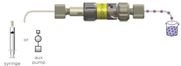
A quick rinse step prior to the elution step is advantageous if salts are present in the sample matrix. Elution takes place either by manual delivery of solvent or by installing the trap cartridge into a holder in-line upstream from an analytical column or within an injection loop.
