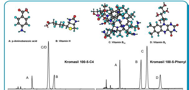
Figure 4. Comparison of Kromasil 100-5-Phenyl to Kromasil 100-5C4. Mobile phase: ACN/20 mM NH<sub>4</sub>H<sub>2</sub>PO<sub>4</sub>, 12/88. Flow: 1.0 mL/min, Wavelength: 210 nm.
