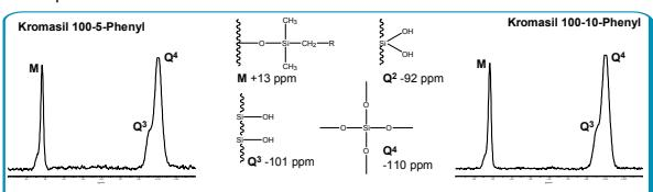
Figure 2.  $^{29}\text{Si}$  CP/MAS NMR of Kromasil Phenyl.
