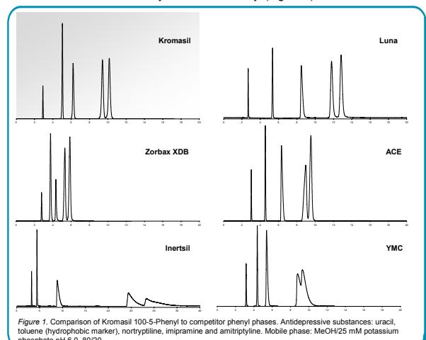
Figure 1. Comparison of Kromasil 100-5-Phenyl to competitor phenyl phases. Antidepressive substances: uracil, toluene (hydrophobic marker), nortryptiline, imipramine and amitriptyline. Mobile phase: MeOH/25 mM potassium phosphate pH 6.0, 80/20.
