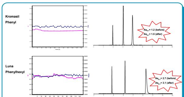
Figure 3. Stability study at pH 9.0 (MeOH/10 mM NH<sub>4</sub>Ac, 80/20) for 6 days. Retention time (Rt) and Plates (N) were monitored for toluene, and the chromatograms shows uracil, toluene and nortryptiline at pH 6.0 after the stability study.
