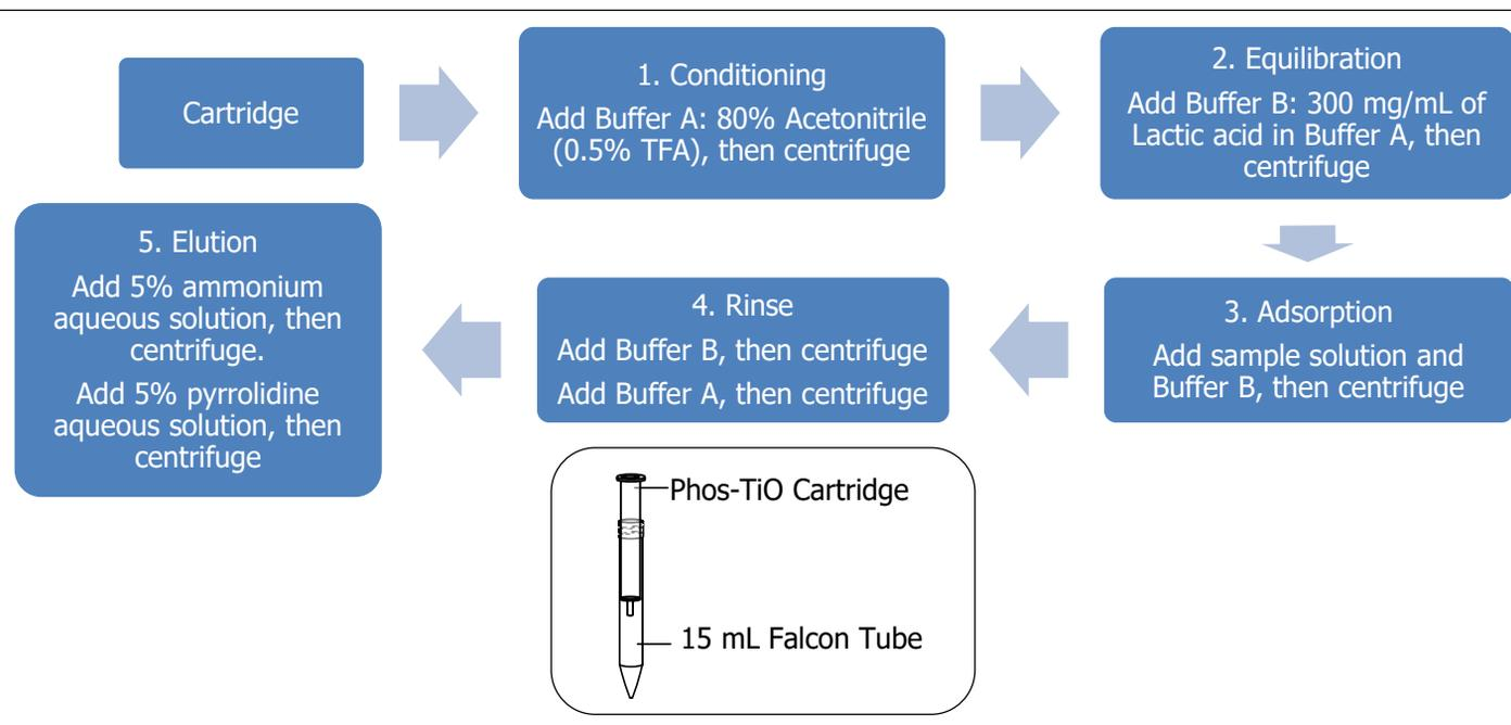
Phos-TiO for Large Volume Samples Cartridges are intended for use with a desktop or other centrifuge. While some of the versions of Phos-TiO resemble pipette tips or SPE cartridges, these products are not intended for use with pipettes or SPE vacuum manifolds; the cartridge internal configuration and particle size of the TiO bulk media requires centrifugal elution of all solutions.
