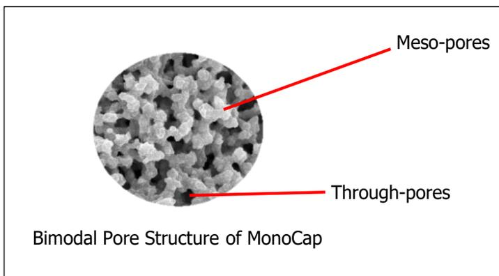
MonoCap HighResolution 2000 is a 2 meter length monolithic silica capillary column which is designed for identifying extremely high number of peptides/proteins for proteome research via LC-MS/MS.
