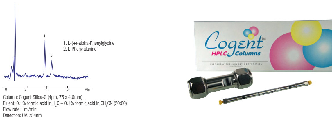
Figure 15. Separation of aromatic amino acids
