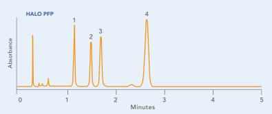
This separation of neutral aromatic compounds illustrates the differences in selectivity between HALO PFP and HALO C18. The  $\pi\text{-}\pi$  interactions offered by the PFP phase and the stronger hydrophobic interactions of the C18 phase lead to significant differences in band spacing and even peak elution order on the two phases. This difference in selectivity makes HALO PFP an extremely useful alternate selectivity to the HALO C18 phase that should be evaluated when developing separations.
