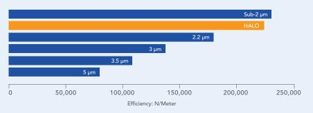
HALO columns deliver over 90% more separating power (theoretical plates) than columns of the same length packed with  $3.5~\mu m$  particles and almost three times the separating power of columns packed with  $5~\mu m$  particles.
