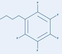
Pentafluorophenylpropyl is the bonded phase used for HALO PFP.
