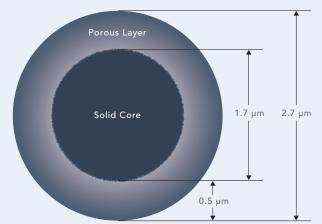
Fused-Core particle technology was conceived of and developed by Dr. Jack Kirkland to produce HPLC columns that deliver UHPLC performance with conventional HPLC equipment. As the name implies, Fused-Core particles are manufactured by fusing a porous silica layer onto a solid silica particle.
