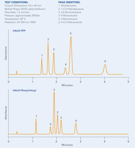
These comparison chromatograms clearly show the effect of different mechanisms of separation: dipole-dipole interactions more dominant with the PFP phase and  $\pi\text{-}\pi$  and hydrophobic interactions more dominant with the Phenyl-Hexyl phase. These differences in interaction between analytes and stationary phase can be utilized to achieve superior separations.
