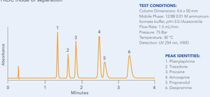
Highly polar compounds that are poorly retained in reversed phase mode can be strongly retained on HALO PFP using HILIC mode. HILIC often provides higher sensitivity for LC-MS applications due to the higher concentration of organic component in the mobile phase.
