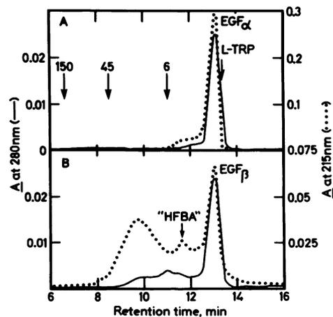
FIG. 5. Size-exclusion chromatography of EGF- $\alpha$  (A) and EGF- $\beta$  (B) on TSK3000SW. Proteins were separated at ambient temperature and a flow rate of 1 ml/min on a TSK3000SW column using 0.1 M phosphate buffer (pH 6.5) and detected by UV absorbance at 280 nm (—) or 215 nm (---). (Only one-fourth the amount of EGF- $\beta$  was used to obtain the 215-nm profile.) (The peak labeled "HFBA" is an impurity in the  $C_3F_7COOH$ .)  $\downarrow$ ,  $M_r \times 10^{-3}$ .
