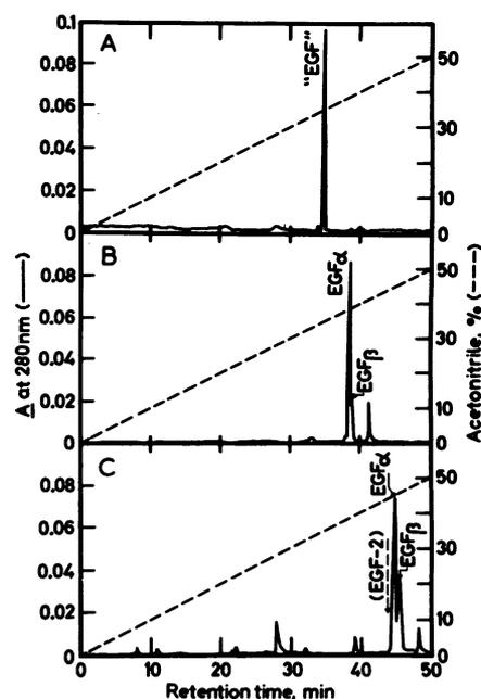
FIG. 1. Comparison of solvent systems for RP-HPLC separation of EGF. Proteins were separated on 15 cm  $\times$  4.6 mm (i.d.) columns of Ultrasphere ODS at ambient temperature and a flow rate of 1 ml/min. Gradient elution was between a primary solvent of 0.1 M sodium phosphate (pH 2.1) (A), 0.2% CF<sub>3</sub>COOH (B), or 0.2% C<sub>3</sub>F<sub>7</sub>COOH (C) and acetonitrile (---). Detection was by UV absorption at 280 nm.
