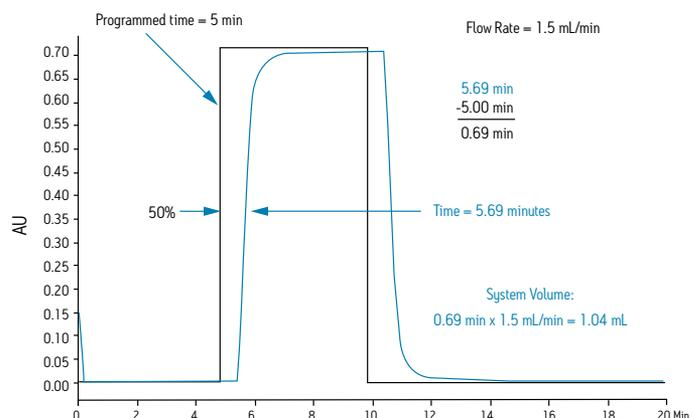
Figure 9: Determination of Gradient Delay Volume
