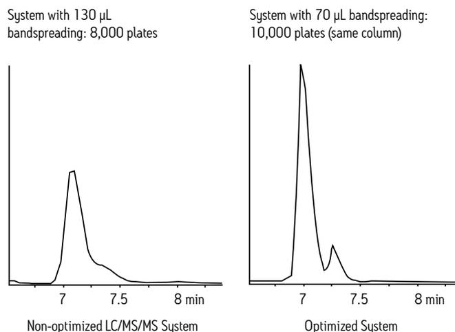
Figure 10: Non-Optimized vs. Optimized LC/MS/MS System
