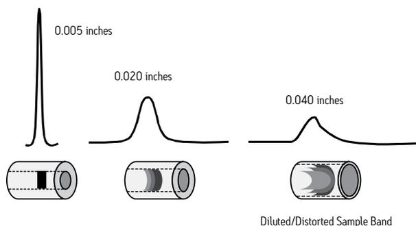
Figure 6: Effect of Connecting Tubing on System
