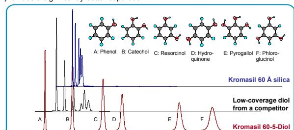
Figure 1. Comparison between Kromasil 60-5-Diol, a low-coverage diol from a competitor, and bare silica, in the separation of six different phenols. Mobile phase: n-heptane/IPA 85:15; Flow rate: 2 mL/min. Detection: UV, 224 nm.
