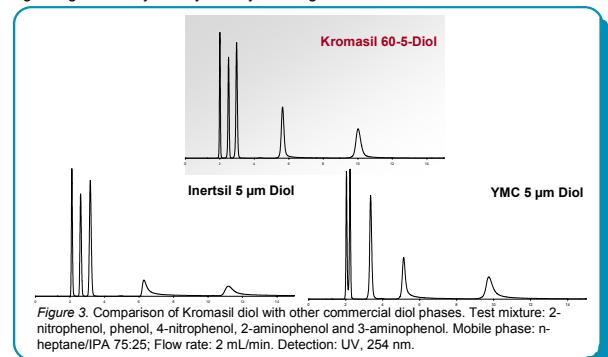
Figure 3. Comparison of Kromasil diol with other commercial diol phases. Test mixture: 2-nitrophenol, phenol, 4-nitrophenol, 2-aminophenol and 3-aminophenol. Mobile phase: n-heptane/IPA 75:25; Flow rate: 2 mL/min. Detection: UV, 254 nm.
