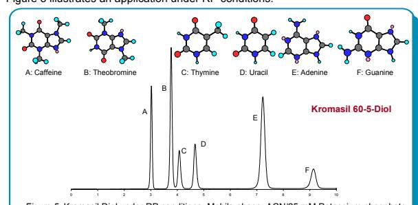
Figure 5. Kromasil Diol under RP conditions. Mobile phase: ACN/25 mM Potassium phosphate buffer, pH 7.85, 80/20. Flow rate: 1 mL/min. Detection: UV, 270 nm.
