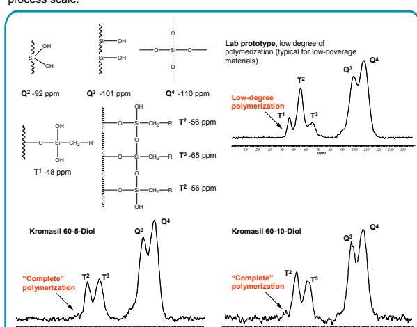
Figure 2.  $^{29}\text{Si}$  CP/MAS NMR of Kromasil Diol compared to a lab prototype with a low degree of polymerization.
