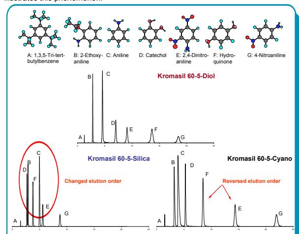
Figure 4. The difference in selectivity for a mixture of anilines and phenols is illustrated for Kromasil Diol, Kromasil Cyano, and bare silica. Mobile phase: heptane/IPA 85/15, Flow rate: 2 mL/min. Detection: UV, 224 nm.
