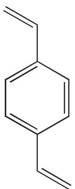
Jordi Gel DVB resin is made from 100% divinylbenzene forming one of the most rugged, hydrophobic packing materials available. The polymer is stable in all solvents and at extremes of pH (0-14). Polymeric beads provide increased sample loading capacity and have greater retention than common silica C18 or PS-DVB phases. Its highly hydrophobic surface provides excellent retention for many compounds of interest in environmental applications.
