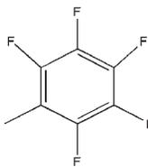
Jordi Fluorinated resin is a 100% divinylbenzene phase with a surface coating formed with fluorinated benzene rings. This patented technology provides decreased absorbance as compared to non-bonded DVB surfaces and is a good option for applications where over retention of the target compound prevents convenient elution. Jordi fluorinated resins are stable in a wide range of solvents and over the complete pH range (0-14).
