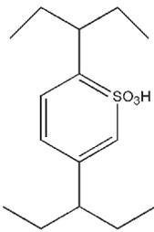
Jordi Gel SCX resin is a water wettable sulfonate modified divinylbenzene polymer. The media exhibits both reverse phase and ion exchange retention for a wide range of basic and neutral compounds allowing easy method development. The phase is stable over the complete pH range (0-14) and can be used with nearly any solvent allowing the use of a wide range of mobile phases. This phase shows excellent retention for essentially all of the common basic drugs of abuse.
