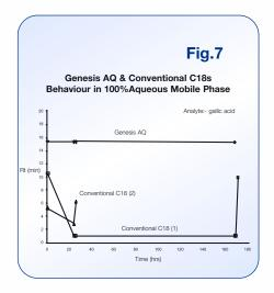
Genesis AQ can be used in up to 100% aqueous mobile phases without the ligand folding or non-wetting of traditional long chain, aliphatic stationary phases such as C18. This effect leads to a reduction in analyte retention time and often poor peak shape. Fig.7 shows this effect for two conventional C18 columns prone to this effect compared to the "inert" Genesis AQ.
