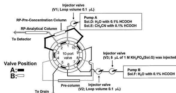
Fig. 2 Schematic diagram of the capillary-sized column-switching HPLC system.
