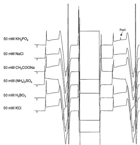
Fig. 4 Evaluation of the influence of the solvent for the elution of phosphopeptides from the titania column.
