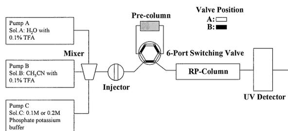
Fig. 1 Schematic diagram of the column-switching HPLC system.
