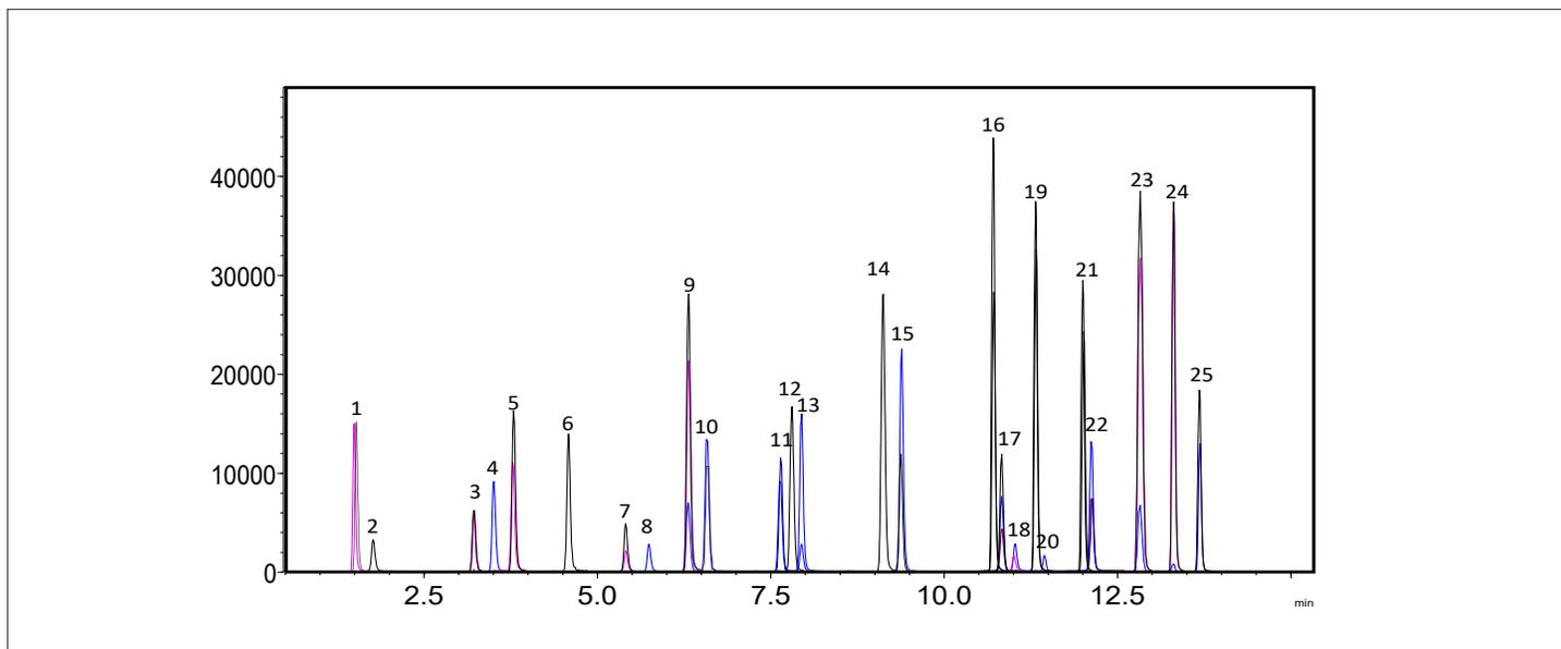
Figure 2. 25 target PFAS compounds specified by EPA 533 separated on the HALO® PFAS Delay and HALO® PFAS columns.
