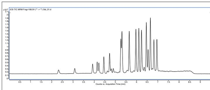
Figure 4 shows the effectiveness of the HALO® PFAS delay column by impeding the instrument PFOA contamination from the sample by 0.7 minutes.
