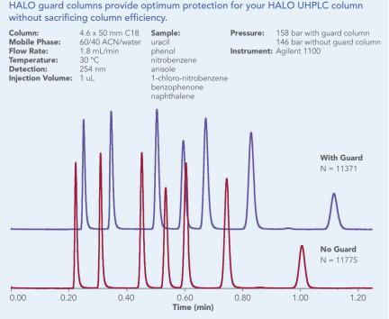
A HALO guard column installed on a HALO C18, 4.6 x 50 mm UHPLC column causes less than a 4% loss in efficiency compared to a HALO UHPLC column with no guard column installed. Since resolution changes with the square root of the change in efficiency, the HALO guard column affects the resolution between peaks by less than 2%.
