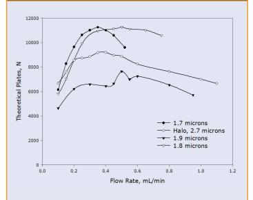
Sample Loading Study: Totally Porous vs. Fused-core Columns: Ascentis C18 and HALO C18, 150 × 4.6mm Detection: 214 nm; Temperature 60°C; Injection: 5μL Mobile Phase: A=20 nm KH<sub>2</sub>PO<sub>4</sub>, pH2.7; B=20nM KH<sub>2</sub>PO<sub>4</sub>, pH 2.7 in 35:65 v/v water/methanol; A : B = 30:70 v/v
