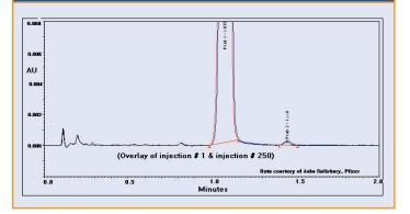
Column Comparison Study with Virginiamycin (MW=574) Ascentis C8 (3.1 µm) ; HALO C8 and HALO C18 (2.7 µm) Columns: 50 x 4.6 mm; Temperature: 30°C; Agilent 1100 Mobile phase: 35% ACN/65% potassium phosphate buffer, pH 3.0
