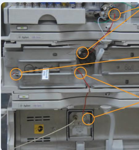
**Step 1:** Replace capillary tubing from sample injector valve to heat exchanger (3  $\mu$ L) in the column compartment.
