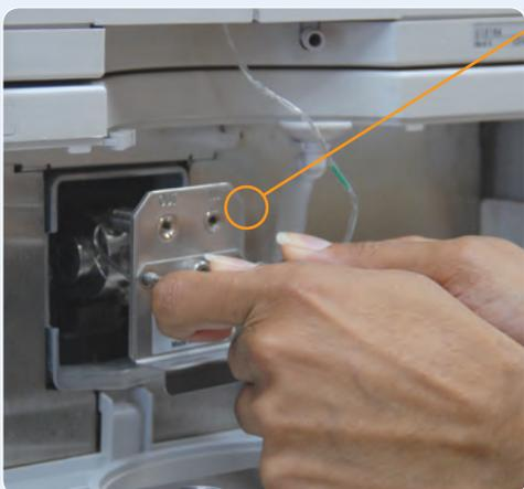
**Step 5:** Remove standard detector flow cell and replace with a semi-micro flow cell or a micro flow cell.
