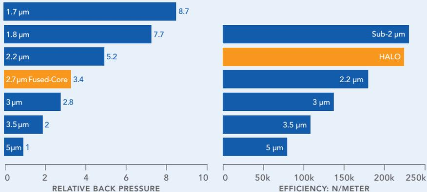
HALO columns packed with Fused-Core particles provide over 80% of the efficiency (theoretical plates, N) and 90% of the resolving power of sub-2- $\mu\text{m}$  columns, but require less than half the back pressure. This lower pressure permits HALO columns to be used with conventional 400 bar-limit HPLC equipment and achieve speed and resolution very similar to UHPLC.
