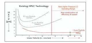
This presentation of data (as seen in *Figure 4*) can mislead the chromatographer into believing that they themselves will see large improvements in their chromatography simply by switching to a sub 2 $\mu$ m column. Whereas in reality each Van Deemter plot is specific to the set of conditions, column geometry and instrument used to generate the data, yet no mention of this is made by those presenting the information.
