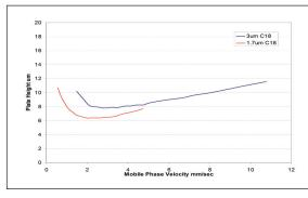
Figure 5b. Van Deemter Agilent 1200 System Result
