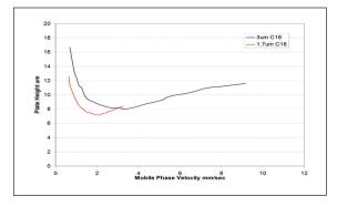
Figure 5a. Van Deemter Agilent 1100 System Result
