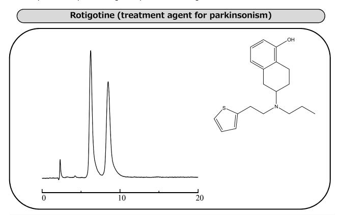
Column: ULTRON ES-OVM (5 µm) 25°C Column temp.: UV-225 nm Column size: 150 mm L x 4.6 mm I.D. Detection:
