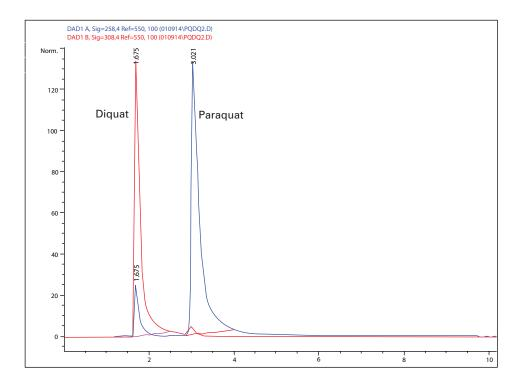
Instrument: HP 1050 Detector: HP Photo Diode Array Column: Selectra® PFPP, 100 x 2.1 mm, 3 μm (UCT p/n SLPFPP100ID21-3UM) Flow Rate: 0.2 mL/min Injection Volume: 1 μL Mobile Phase A: 10mM Ammonium Acetate (pH=4) Mobile Phase B: Acetonitrile Isocratic: A:B (99:1) Monitoring Wavelength: Diquat: 308 nm Paraquat: 258 nm
