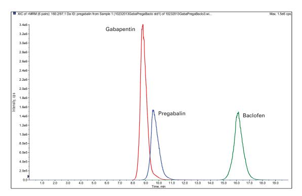
Instrument: Agilent 1200 Binary Pump SL Detector: ABSciex 4000 Qtrap MS/MS Mode: ESI + Column: Selectra® PFPP, 100 x 2.1 mm, 5 μm (UCT p/n SLPFPPID21-5UM) Flow Rate: 0.5 mL/min Column Temp: 50 °C Injection Volume: 10 μL Mobile Phase A: 0.1% Formic Acid in H<sub>2</sub>O Mobile Phase B: 0.1% Formic Acid in MeOH Isocratic: A:B (85:15)
