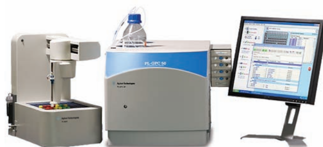
The Agilent PL-GPC 50 Integrated GPC/SEC System with autosampler on the left, display on the right and solvent pump, column oven and detector in the housing in the middle
