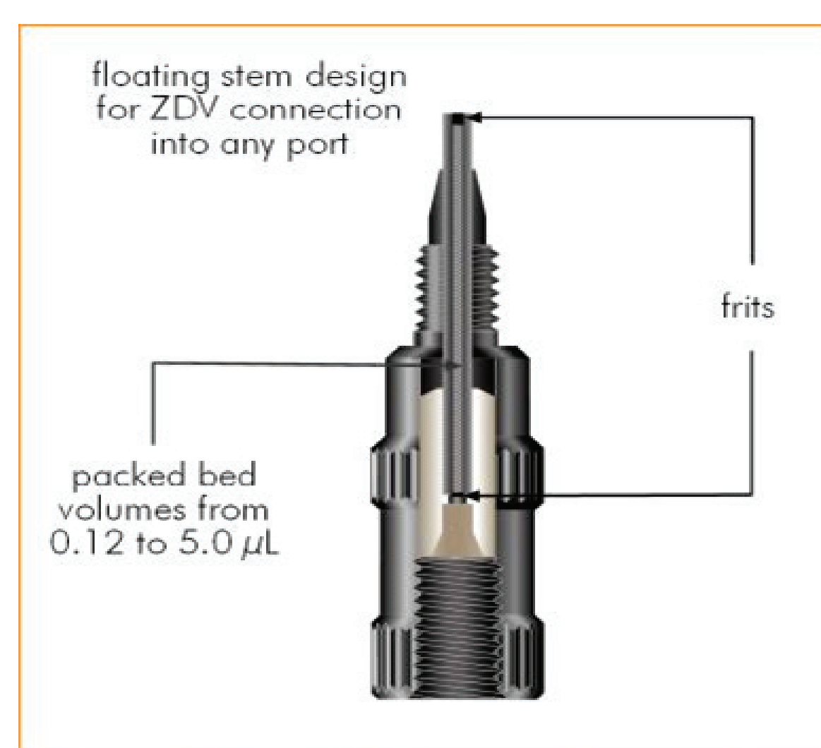
Figure 1 Diagram of new OPTI-PAK® design with packed bed directly in stem tube.
