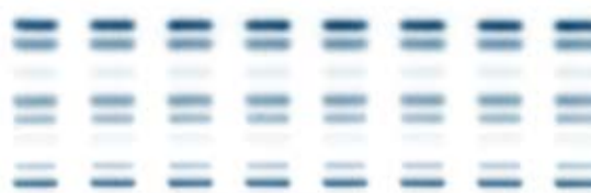
Merck Millipore TLC plates deliver highly reproducible sharp bands over the whole plate as demonstrated by the parallel separation of a lipophilic dye mixture on a silica gel 60 classical TLC plate
