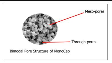
MonoCap HighResolution 2000 is a 2 meter length monolithic silica capillary column which is designed for identifying extremely high number of peptides/proteins for proteome research via LC-MS/MS.
