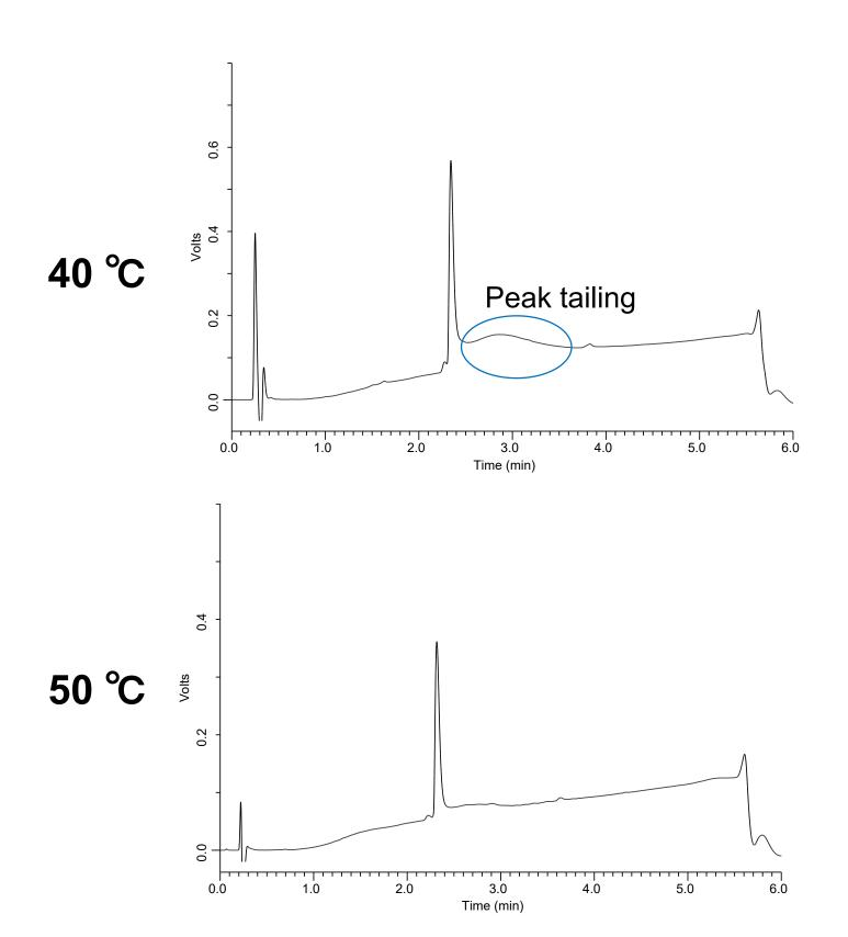
Separation of Intact mAb using a developed monolithic column at different temperatures.
