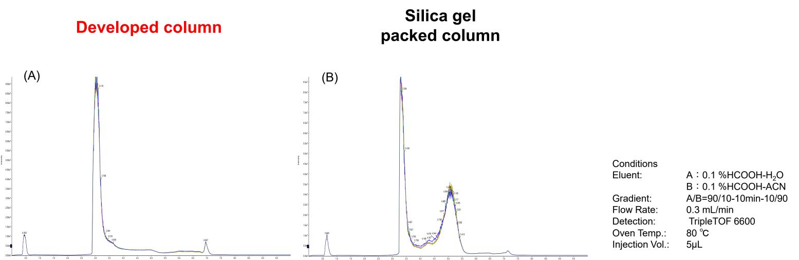
Intact mAb mass analysis (total ion chromatogram) on (A) an developed column, (B) silica packed column.
