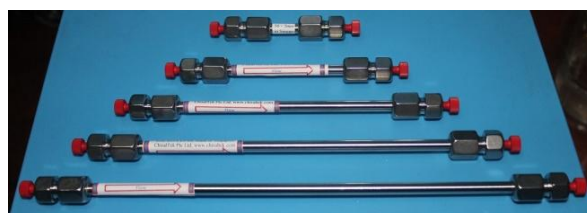
Figure (B). Typical photo of the ChiralCD-1 columns with different length
