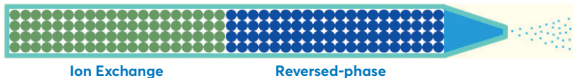
Figure 49. Multidimensional Protein Identification Technology (MudPIT) consists of an initial fractionation of a protease digestion of an entire proteome by ion exchange chromatography followed by a lengthy reversed-phase separation of the peptides from each fraction of the ion exchange separation. Narrow capillaries are packed with ion exchange beads and reversed-phase beads and the eluent from the chromatography is directed into an electrospray mass spectrometer.
